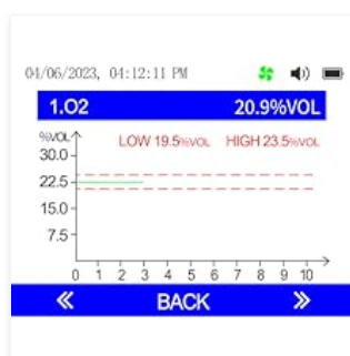
Figure 5.3: The 'View curve' screen, illustrating the historical trend of gas concentrations, such as O2 levels, relative to alarm thresholds.
